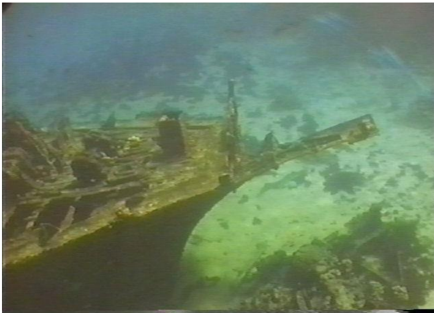
Site 3 Photo 1. The bow of the vessel Seisho Maru. Note part of the bow spirit has fallen away. The chain comes out of the port side chain locker and out the port side tube to the anchor. There was no starboard side anchor or chain.
