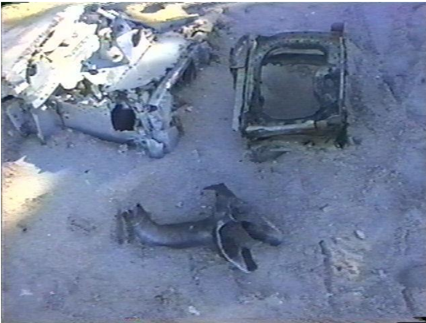
Site 2 Photo 5. Section of wing from this aircraft was washed towards shore and rests within the sandy beach. An unknown fuselage section is in the upper right, and an exhaust collector segment is in the lower center. The main site is approximately 100 yards away.
