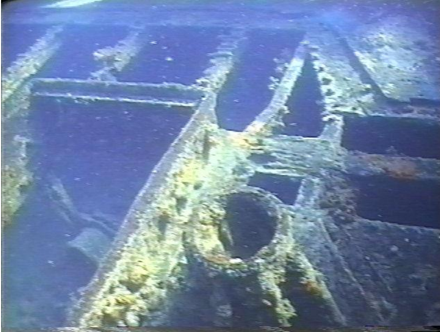
Site 4 Photo 7. The main deck forward had a wooden mast socket, and the larger hatch behind it was used for easy and clean entry into the hold.
