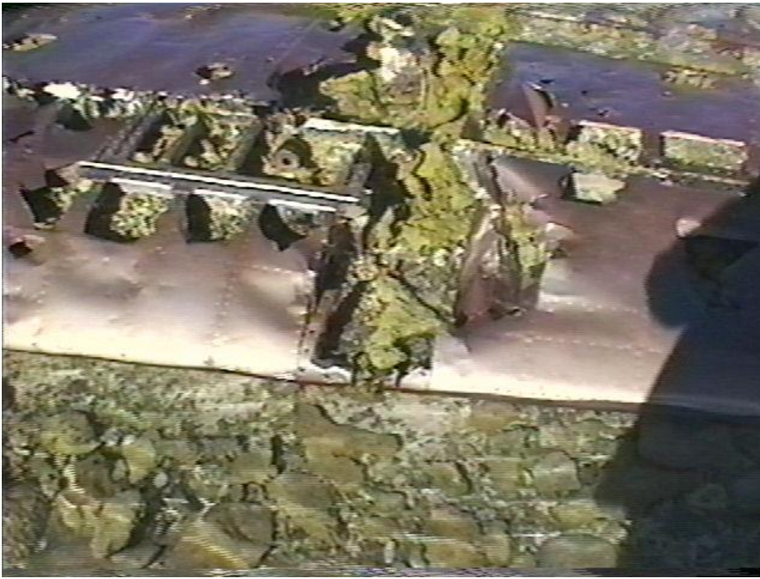
Site 5 Photo 8. Cavity in left wing where 20mm cannon used to reside.
