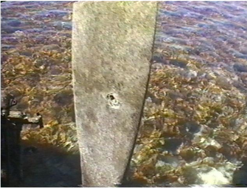
Site 1 Photo 10. A bullet hole in the upright propeller blade is probably from attacking American planes after the aircraft was in the water.
