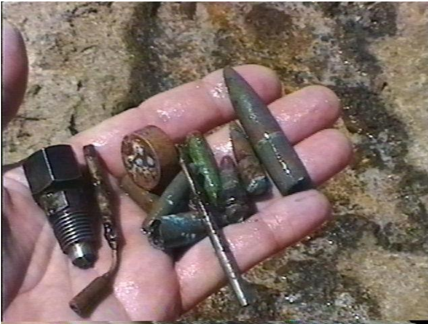
Site 7 Photo 11. Beach objects collected near the north engine from pockets in the reef. Items include, from left to right, a hydraulic/pneumatic fitting, a brass rod, a stainless rod, a bronze engine injector part, and six brass bullets, either 5.62mm or 7.65mm Japanese rifle rounds, and one .50 caliber US machine gun round on the far right.
