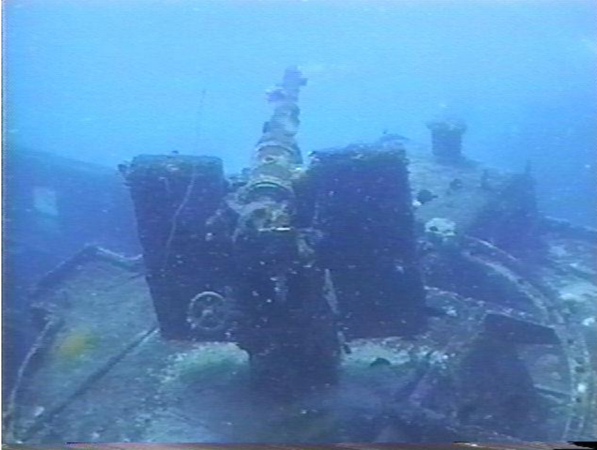
Site 4 Photo 3. The gun mounted on the bow is the prominent feature of the vessel. It probably fired a 40mm round, but no ammunition was found at the site. A ready ammunition locker generally sat nearby.
