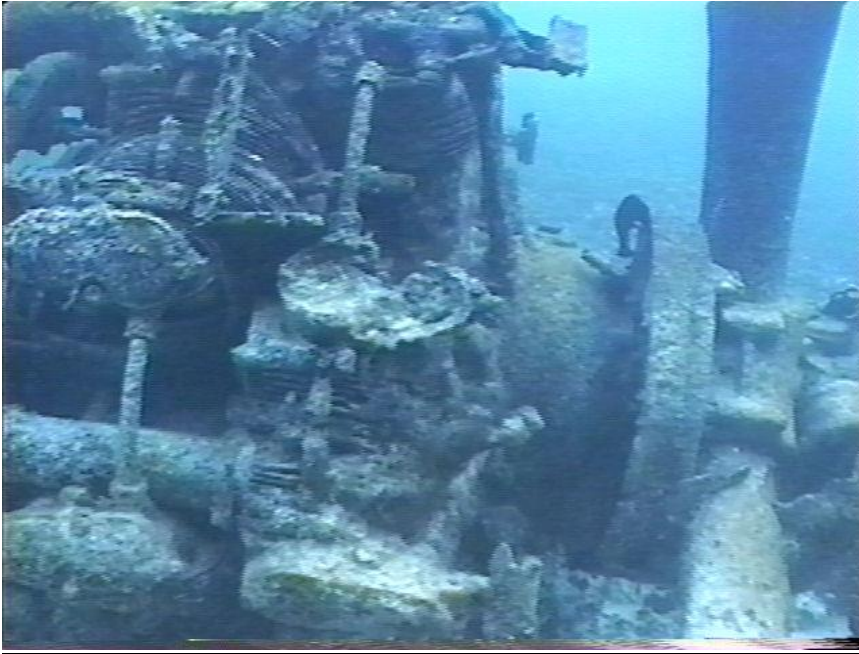
Site 1 Photo 3. Close photo of right side of Sakae engine. No cowling survived, but the blades are still in place.
