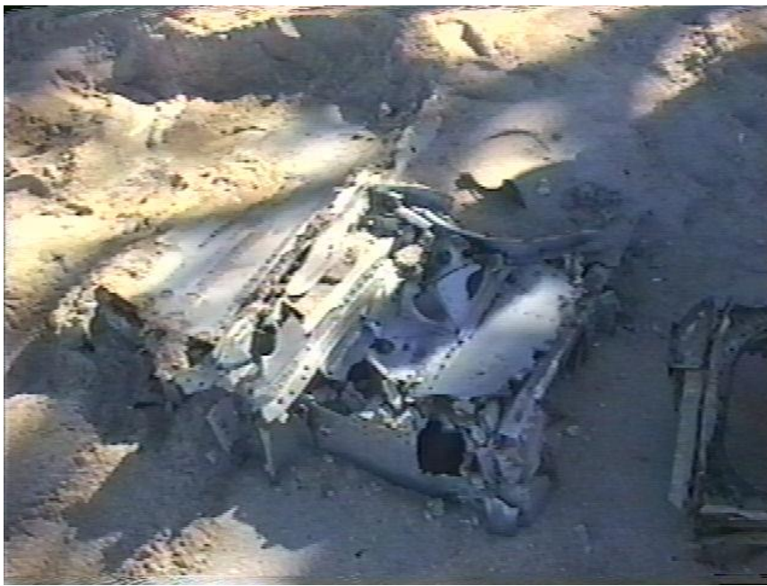
Site 2 Photo 3. A section of the left wing of the Central Ollet A6M lies partially buried in the sand at low tide. It has torn off at the landing gear area.
