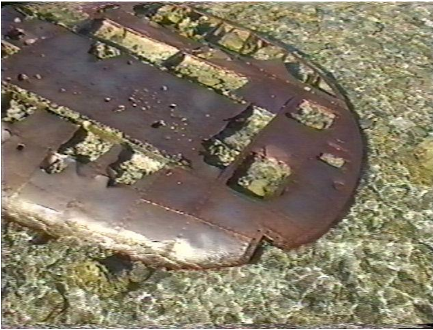
Site 5 Photo 10. Photo of the left wingtip. This is not a folding wingtip; so earlier identification made it an A6M2 Model 11, which was a lighter production model for Imperial Japanese Navy (IJN) shore based units. As many variants were produced, and field modifications made, it would take a true aircraft expert to determine the exact model.
