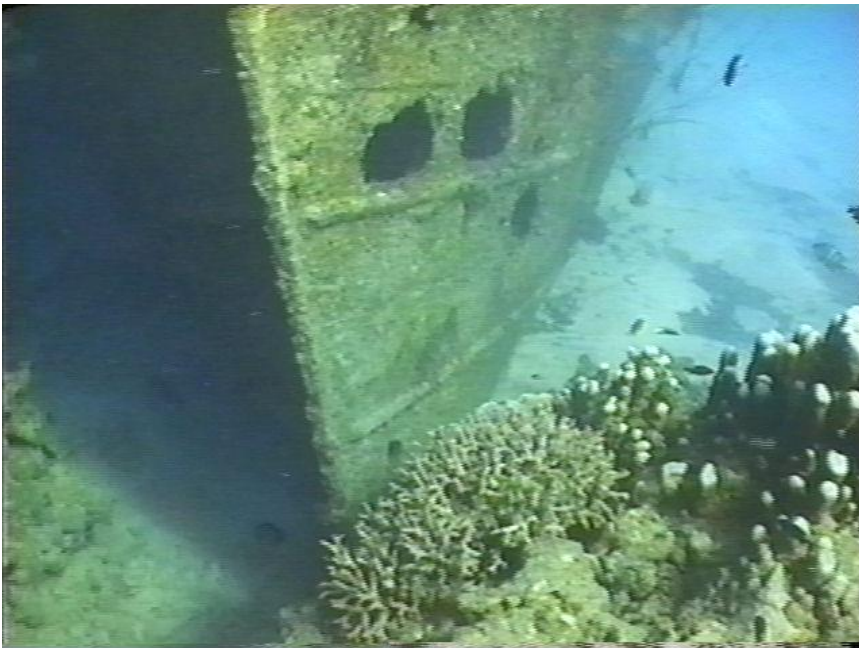
Site 4 Photo 2. The holes in the bow were probably created by corrosion over time, and not by the effects of war. This was the “wind and water line” area of the vessel, which decays the fastest.
