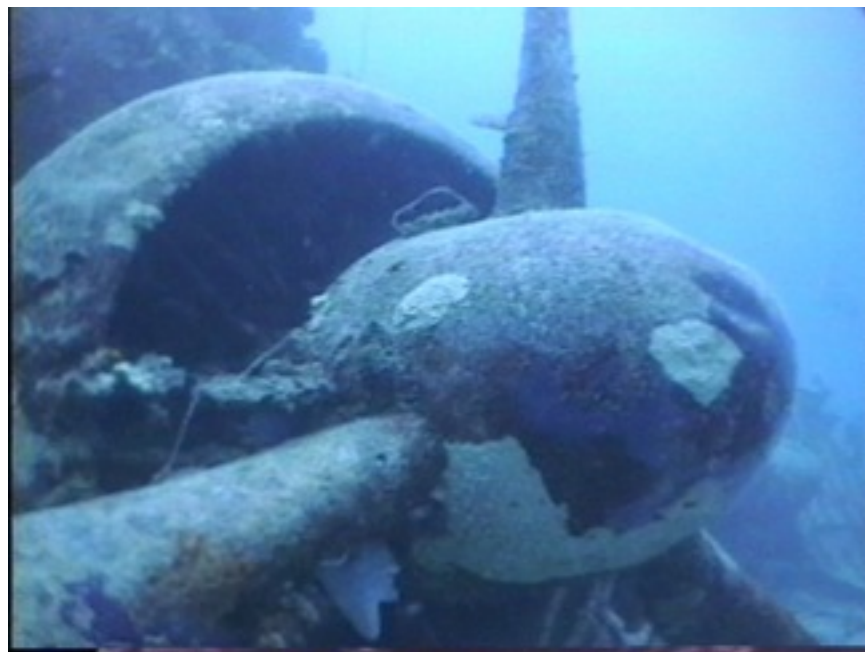
Photo KS5-3 The only engine still attached to a wing section on the North Mavis Flying-Boat wreck. Note 3 bladed propeller.
