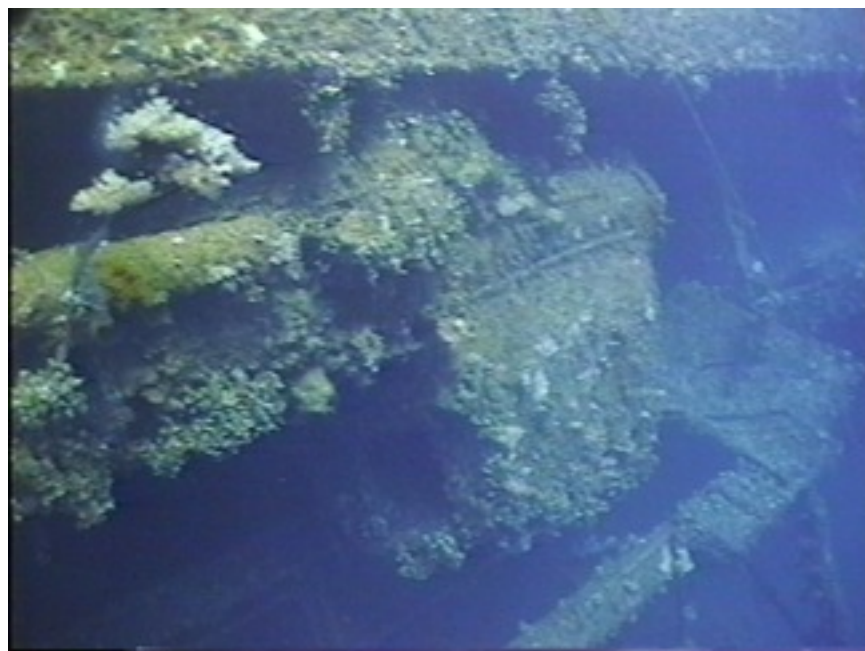
Photo KS13-7 Hanging hull section from damage site. Section is attached to anti-submarine cable and extends almost to the sand.
