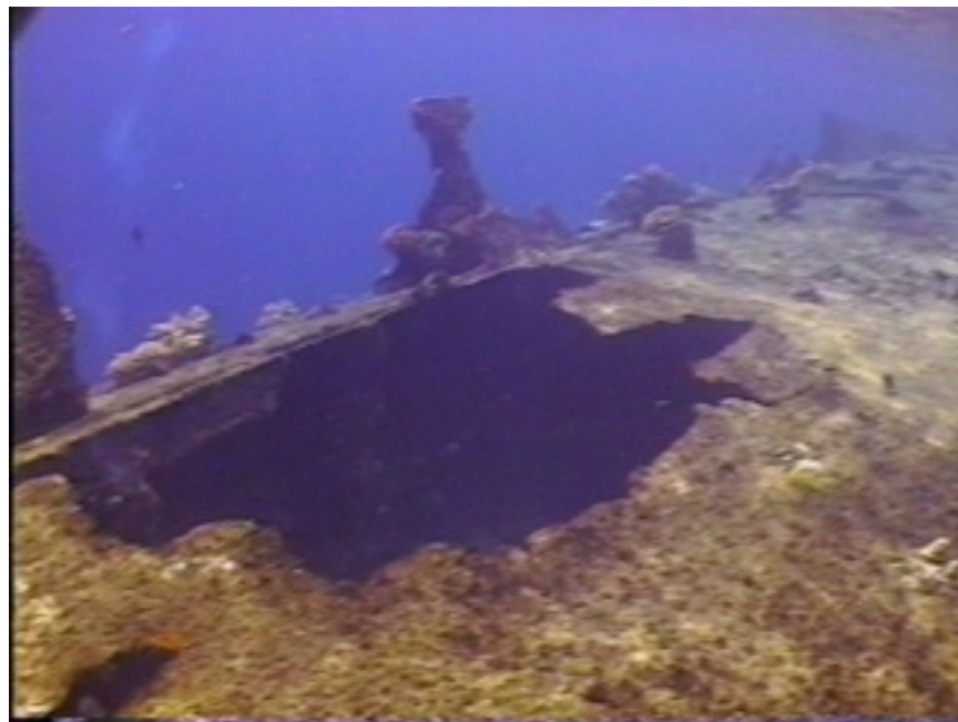
Photo KS13-2 Bottom hull of Prinz Eugen showing port side bilge keel on right of photo and sea chest intake in bottom of photo.
