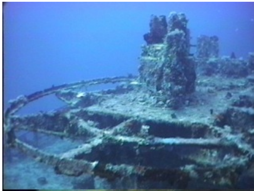
Photo KS10-3 Empty gun mount on bow of Akibasan Maru. Gun was a 75mm model.
