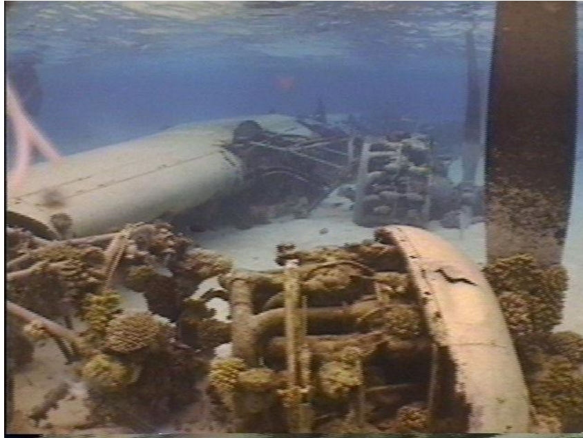
Photo MS1-3 B-24 Engines 3 and 4, slightly separated from original mountings
