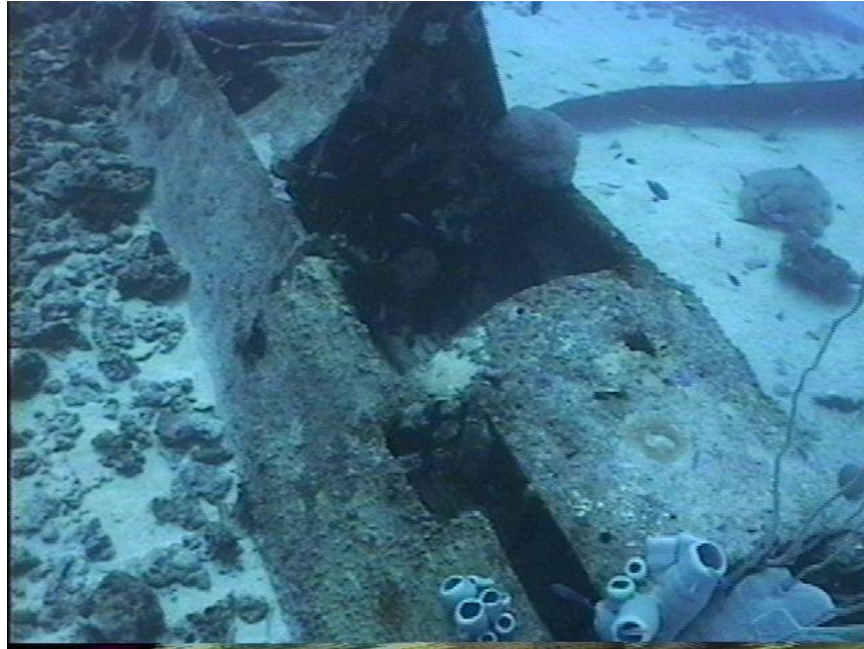
Photo MS2-7 Close up of pilot area. Single machine gun slot on right side is visible, as is armor plate behind pilots head.
