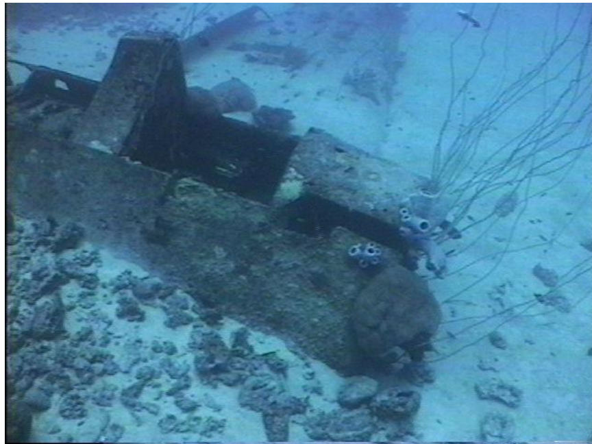
Photo MS2-6 Front of aircraft without engine. Whip coral grows out of firewall area. Note debris on right wing, and left wing is basically clear.
