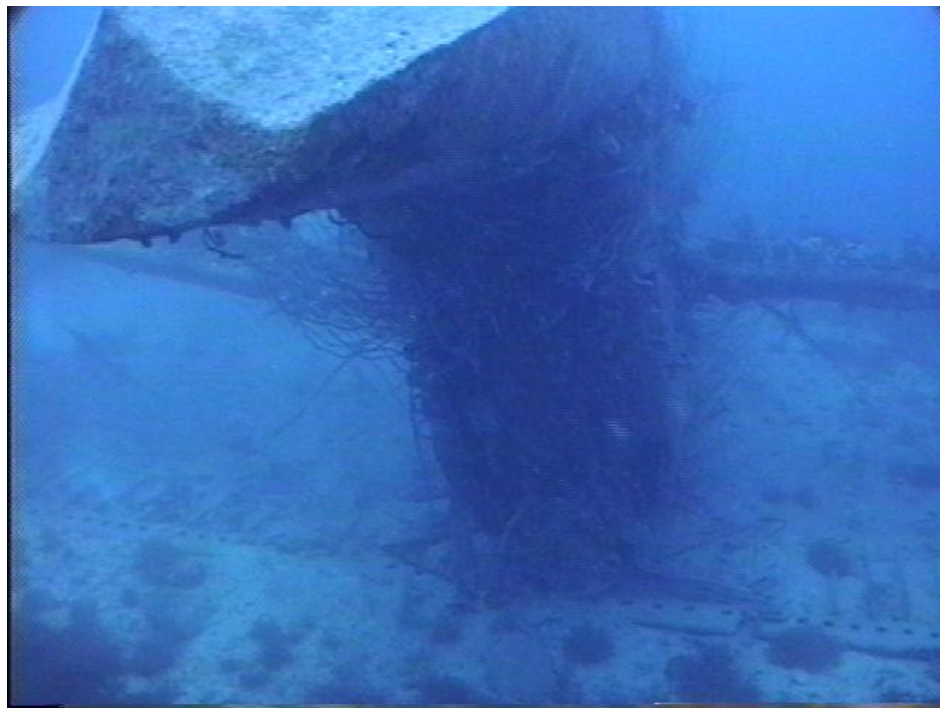
Photo MS10-4 Engine mounting area on Grumman Duck, engine has been removed.
