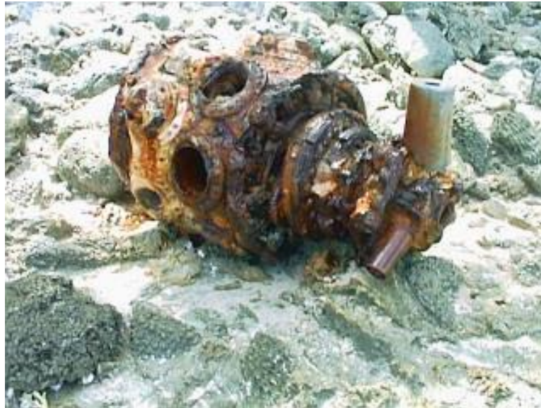
Photo MS2-3 US TBM/TBF "Avenger" engine block assembly on oceanside of Bokollap island. Note hack-sawed off top propeller blade.
