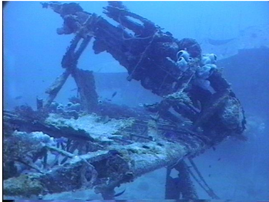
Photo MS10-7 Remains of the pontoon hang on the wing. Other side pontoon has fallen off.
