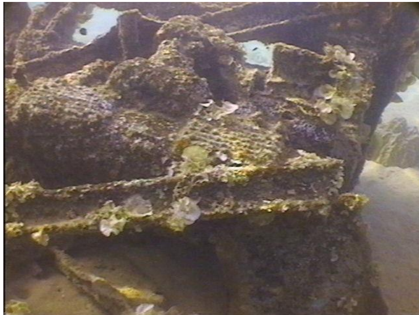
MS8-9 Main engine of the US Navy tugboat near the Majuro Seaplane Ramp. Experts think this was an "Atlas " or "White" 2 cylinder gas engine, made in the late 1930's. ( Eachus, 1999: Oral History ).
