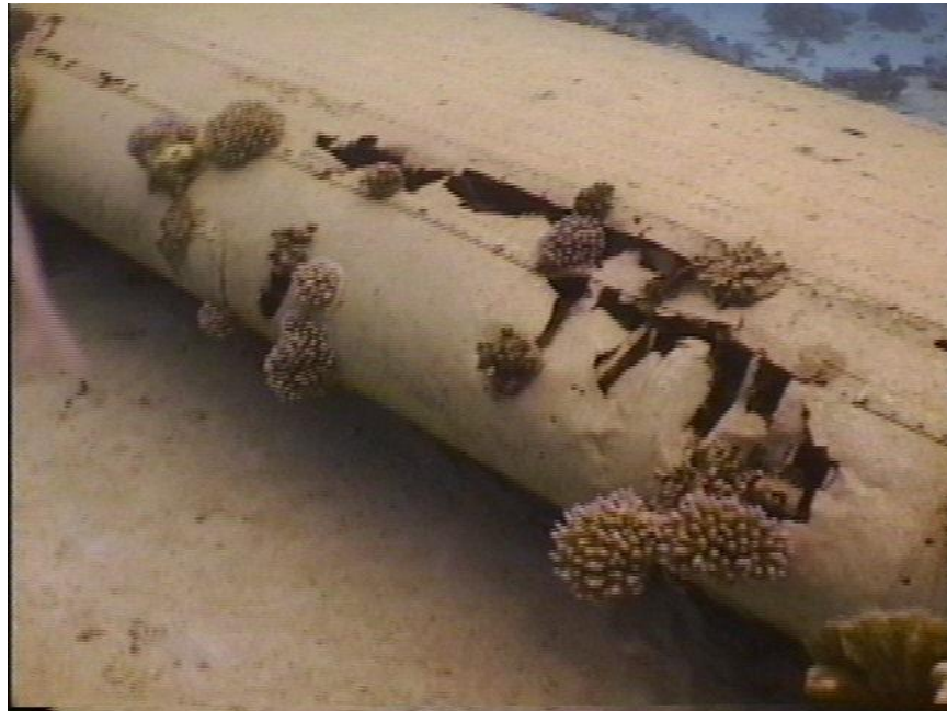
Photo MS1-7 Damage to leading edge of wingtip from unknown sources.
