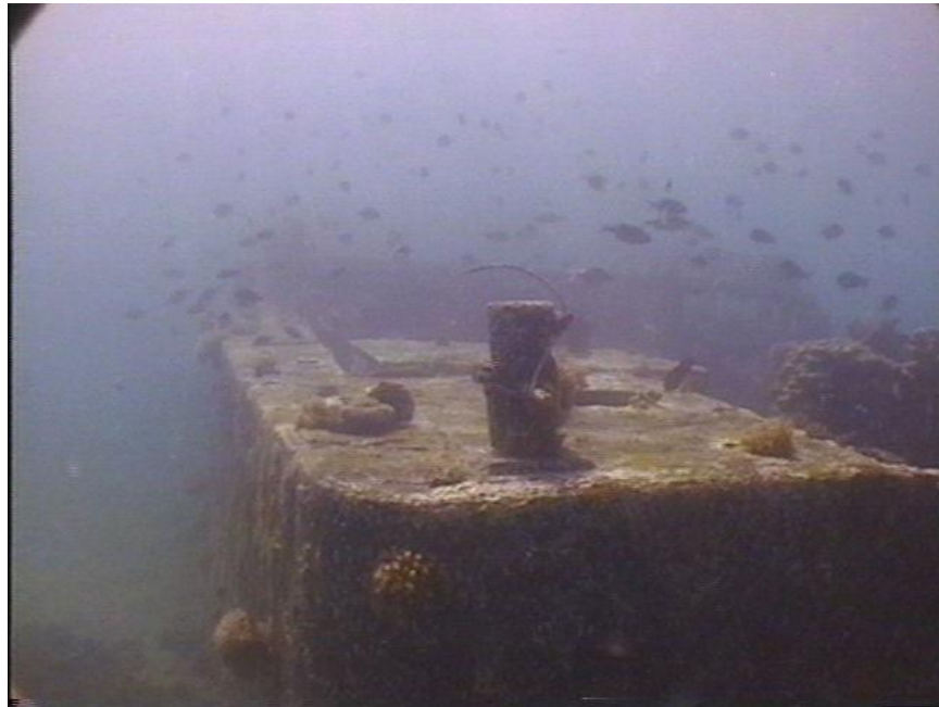
Photo MS7-6 A small landing craft abandoned at the Marine Railway site. Craft identified as a 56 foot LCM, stripped of engines, shafts and propellers.
