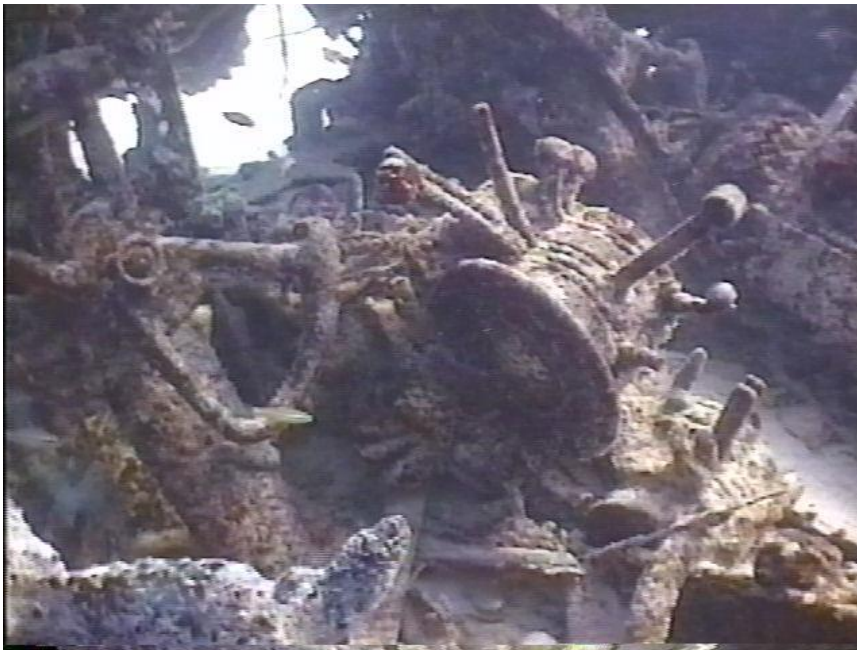
Photo Mi-10-7. Throttle quadrant of the B-25D. Fourth large lever from the right, the pitch control, is pulled back and down away from the others which are pushed all the way to the top of the quadrant, and indicates the right engine was possibly being feathered.
