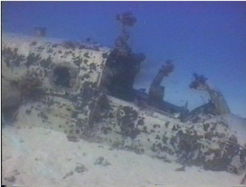
Photo Mi-10-6. Photo of the pilots area, with most glass and 1 pilot seat missing. The mast for radio wire antenna and the base for radio direction finder are visible on the top of the aircraft.
