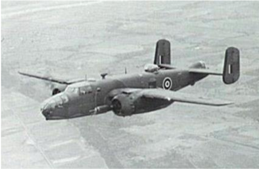
Photo Mi-10-4. Unique photo of an exact Pacific version of a D model B-25, flown in this photo by the RAF. Note single 50 caliber machine gun under the cockpit, plus waist guns mounted forward of the top turret ( Avery, 1992:148 ).
