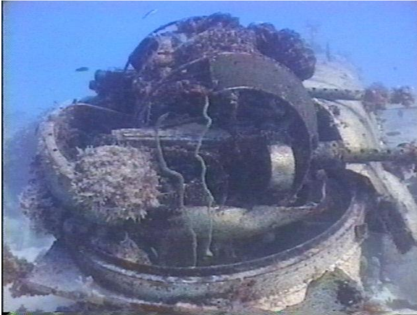
Photo Mi-10-10. Top turret with dual 50 caliber machine guns.
