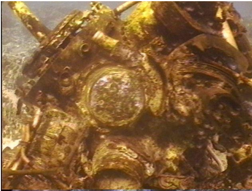
Photo WT1-6. Close-up of Wright Cyclone R 2600 engine of a SB2C "Helldiver".
