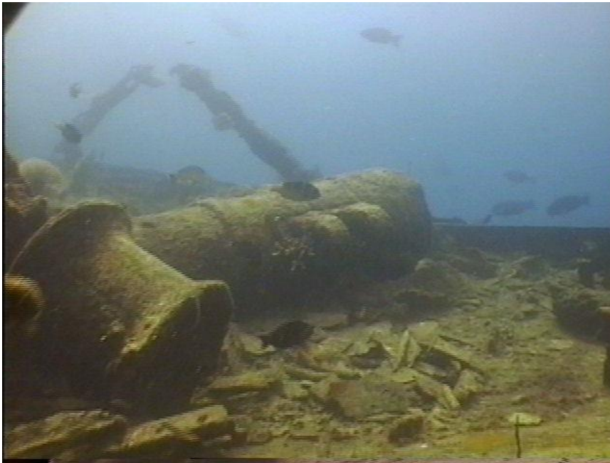
Photo WT13-9. Stern debris, with winch and king-post lying on remains of a section of the port side deck.
