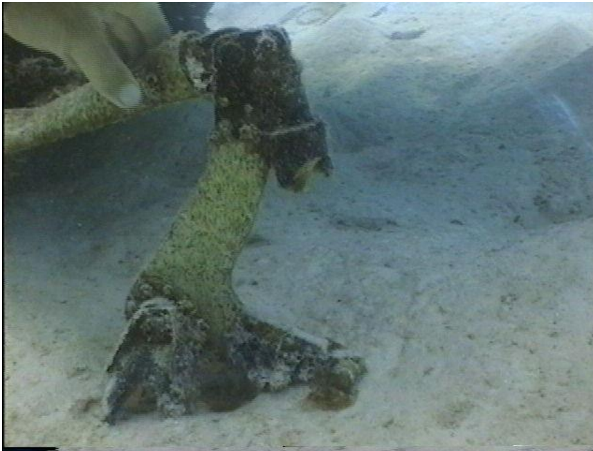
Photo WT8-9. A control arm stuck in the sand, very similar to a control arm for the ailerons for a Mitsubishi G4M "Betty" bomber.
