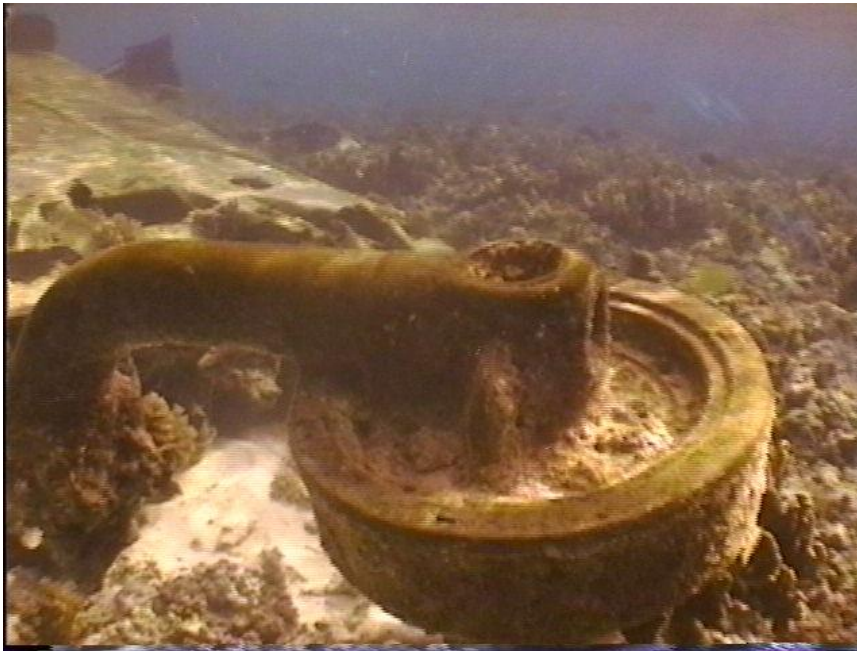
Photo WT1-7. Landing Gear Hub at the end of the severed right wing
