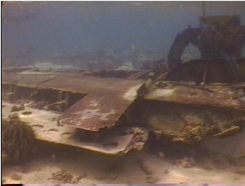
Photo WT1-9. Left wing section to the left of photo, with the remaining fuselage to the right. Note air brakes retracted in left wing assembly.
