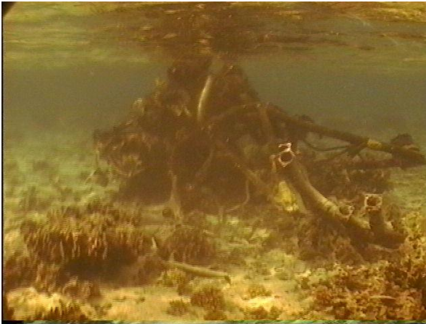
Photo WT1-5. View of entire engine remains of SB2C aircraft. Note bright stainless steel exhaust manifolds in right side of photo.
