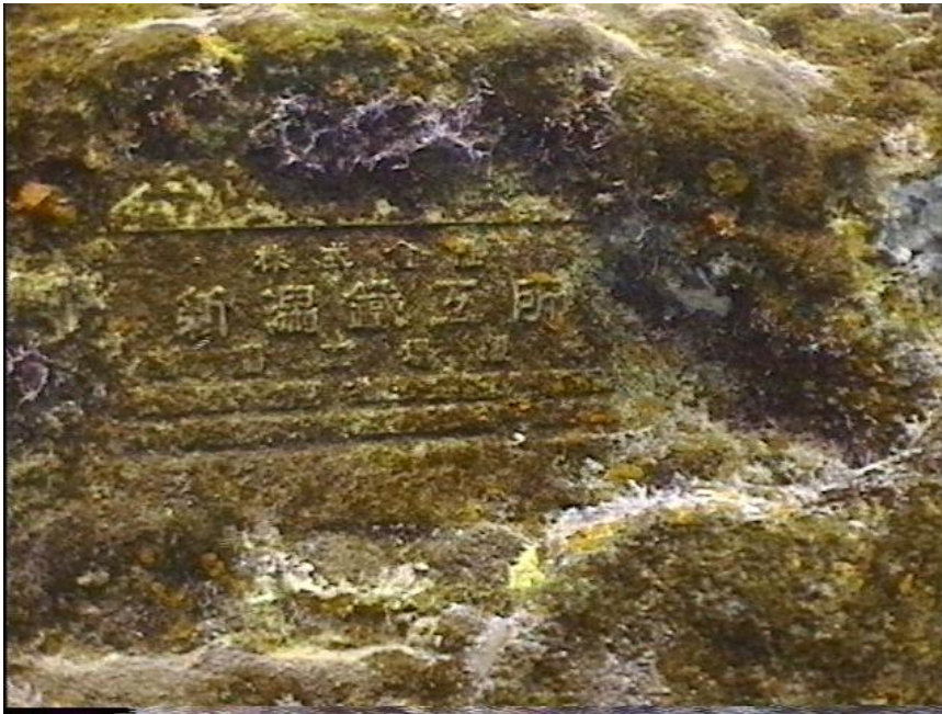
Photo WT7-8. Engine ID plate translating into Niigata built diesel engine.
