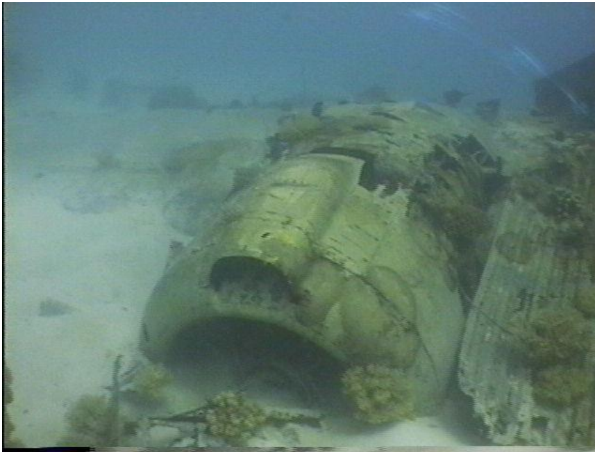
Photo WT5-10. Number 4 engine of the Kawanishi H8K aircraft.
